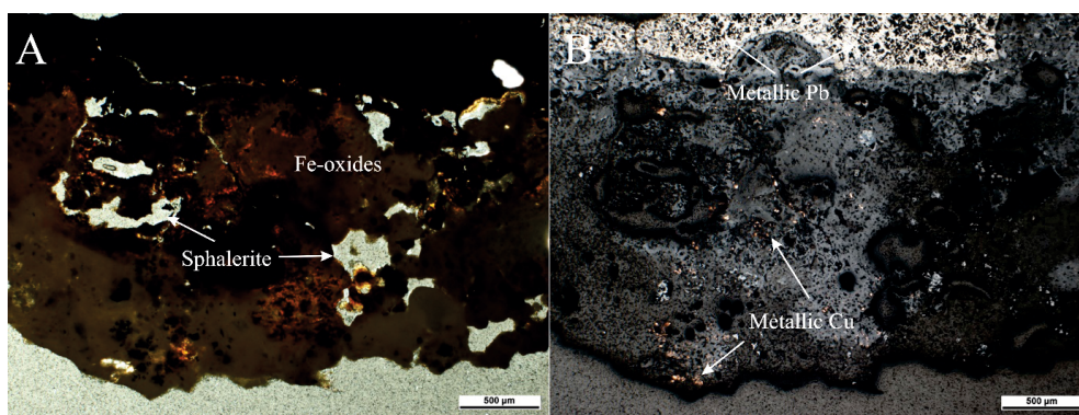
Fig. 3. Slag samples photos from under an optical microscope A) transmitted light; B) reflected light. Magnification \times 2.5
