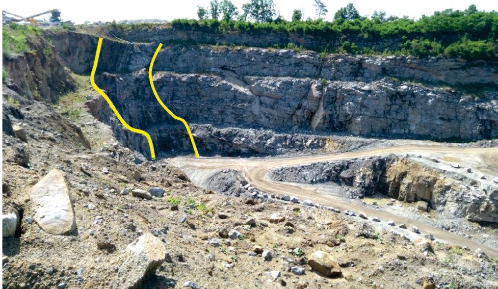
Fig. 1. The eastern part of the Łażany II deposit with the hornfels zone occurrence (between yellow lines)
