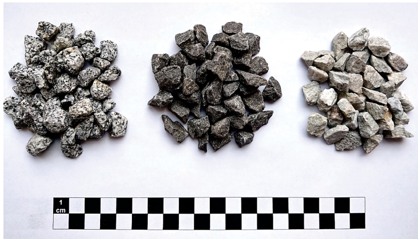
Fig. 2. The groups of samples of selected rock types separated from aggregate with grain size 8/11 populations separated from the general 8/11 aggregate samples, from the left: granodiorite, dark gray hornfels, light gray hornfels with a greenish tinge
