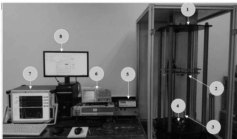
Fig. 4. Mechanical structure and measurement facility: 1 – mechanical structure, 2 – falling mass, 3 – velocity sensor, 4 – force transducer, 5 – charge amplifier, 6 – oscilloscope, 7 – data acquisition system, 8 – computer.
