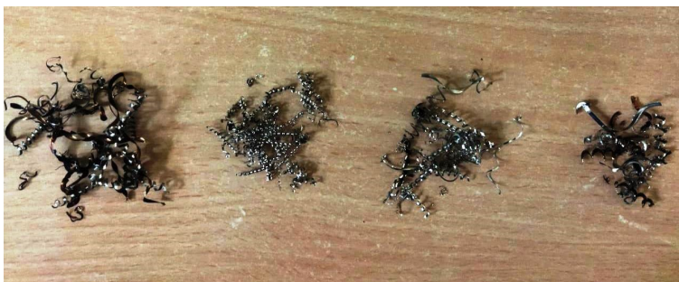
Fig. 1. Chip formation for the cutting speeds 65, 81, 95, and 106 m/min (from left to right)
