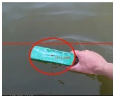
Fig. 7. The Results of Image Processing using HSV Algorithm for Milo Box Garbage
