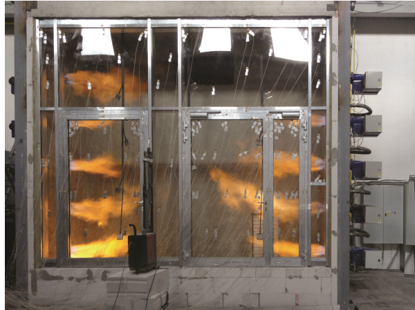
Fig. 2. Aluprof MB-78EI system partition fire resistance laboratory tests
