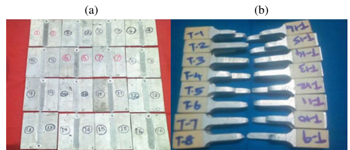
Fig. 1. (a) Welded specimens, (b) tensile specimens after fracture
