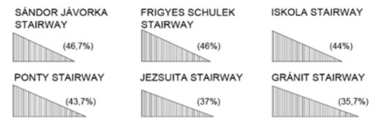
Stairways ranked according to gradient starting from the highest percentage (the whole length of the stairway including stair flights and landings)
