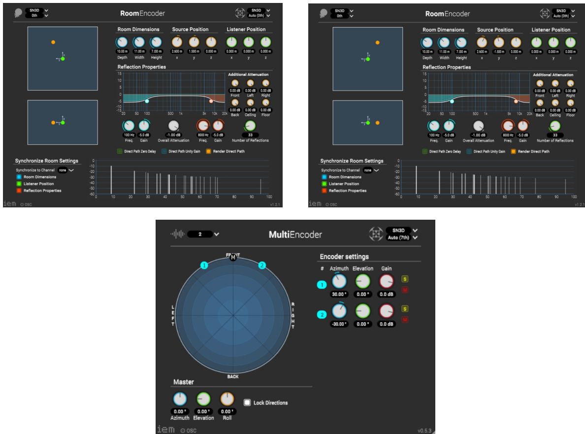
Fig. 3. Example of plugin setup for \pm 30^\circ virtual loudspeaker setup.
