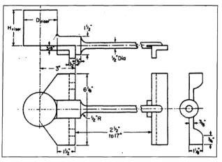
Fig. 12. The flanged bar casting mould design [49]
