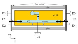
Fig. 28. The new-experimental "T" Shape casting scheme [69]
