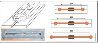
Fig. 16. The hot tearing test with dog-bone mould [52, 53]
