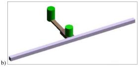
Fig. 27. (a) The schematic of "T" shape casting and (b) The addition of a riser in the centre of the specimen arm [68]
