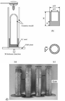
Fig. 37. The illustration of the test scheme for castability using the tube-shaped mould method, (a) an alumina mould with a singlecrystal (SC) seed was used for the growth of the SC or bicrystal (BC) structure, (b) the dimensions of the SC seed, (c) the top view of the cross-section, and (d) the tube-like specimen cast BC [89,90]
