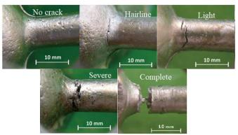
Fig. 6. Typical hot-tearing on the casting surface [43]
