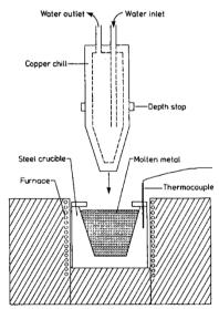
Fig. 19. The chilled casting moulds [55]
