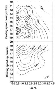
Fig. 4. The effect of casting speed and Cu concentration on the hot cracking (HCS) of Al-Cu alloys [41]
