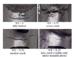
Fig. 5. The WF for various tearing types [42]
