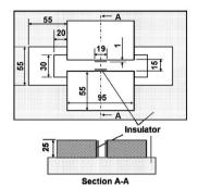
Fig. 35. The I-beam cracking casting test mould [87].
