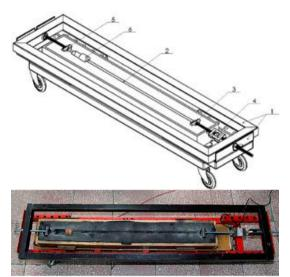
Fig. 26. The test scheme of hot tear tendency, (1) frame, (2) rod sample-sand mould, (3) fixing of the rod end, (4) tensommetric system of force measuring, (5) fixing of the rod stable end, and (6) Thermo insulating insert [66]
