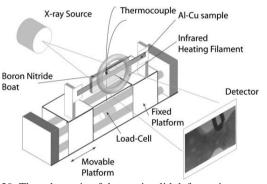
Fig. 39. The schematic of the semi-solid deformation apparatus [93]
