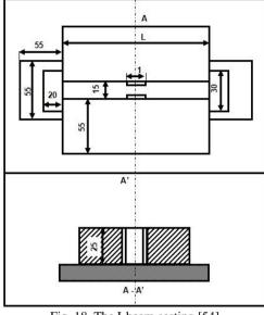
Fig. 18. The I-beam casting [54]
