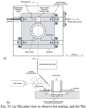
mould cut in sections A-A [82]
