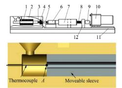
Fig. 36. The schematic of an ARCA instrument with sections, (1) Insulating material, (2) Permanent moulds, (3) Steel bolts, (4)
