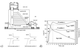
Fig. 21. (a) The Schematic of CRC mould and the measurement of hot tear value, (b) The CRC mould with loadcell, (c) The CRC mould with loadcell and increasing rod numbers, and (e) The load and cooling curves [57,67]
