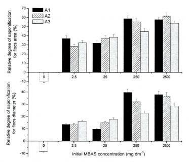
Fig. 1. Comparison of the relative degree of flocs saponification estimated for mean projected area and diameter of flocs in the batch experiments
