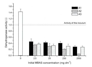
Fig. 3. Comparison of dehydrogenase activity of activated sludge biomass in the batch experiments
