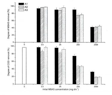
Fig. 4. Comparison of degree of MBAS and COD removal in the batch experiments
