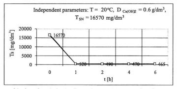
Fig. 3. Influence of the time of gravitational sedimentation  $t_s$  on the concentration of total suspension  $T_s$  in wastewater after coagulation
