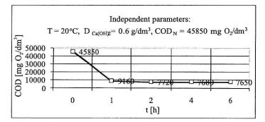
Fig. 6. Influence of sedimentation time  $t_s$  on the COD value in wastewater after coagulation
