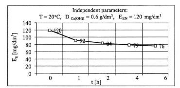
Fig. 9. Influence of sedimentation time t<sub>e</sub> on ether extract value in wastewater after coagulation
