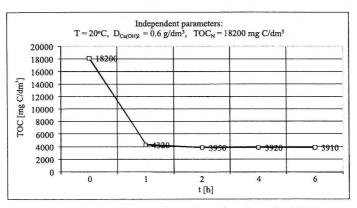
Fig. 12. Influence of sedimentation time  $t_s$  on the total organic carbon value TOC in wastewater after coagulation
