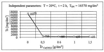
Fig. 2. Influence of Ca(OH), dose on the concentration of total suspension  $T_s$  in wastewater after coagulation
