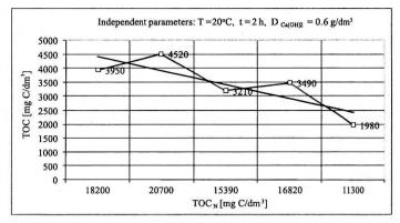
Fig. 13. Influence of total organic carbon value TOC<sub>N</sub> in inflow wastewater on total organic carbon TOC value in wastewater after coagulation
