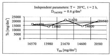
Fig. 4. Influence of the concentration of total suspension in inflow wastewater  $T_{sN}$  on the concentration of total suspension in wastewater after coagulation  $T_s$
