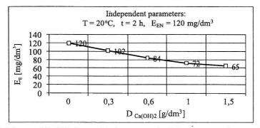
Fig. 8. Influence of Ca(OH)<sub>2</sub> dose on the ether extract value E<sub>1</sub> in wastewater after coagulation
