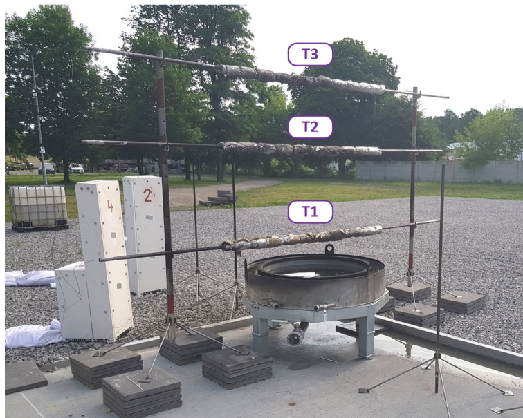
Fig. 1. Pool fire test stand: T1–T3 – thermocouples
