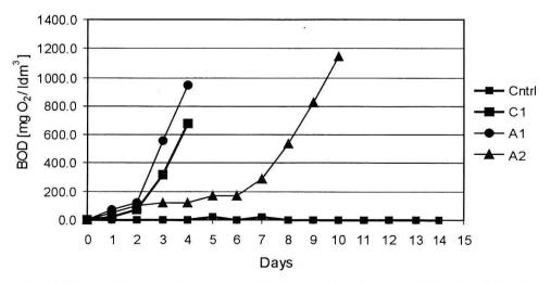
Fig. 2. Changes of biochemical oxygen demand during experiment in seawater during degradation of hydrocarbons
