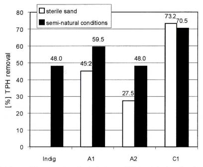
Fig. 3. Influence of bioaugmentation with mixed culture on TPH degradation in sterile and non-sterile sand polluted with 5% of crude oil
