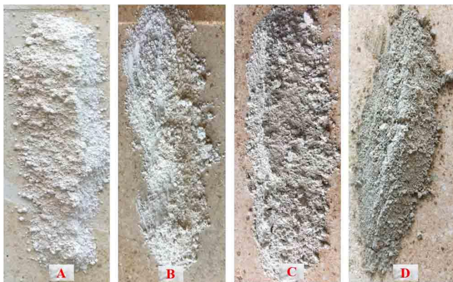
Fig. 3. A) limestone dust before calcination, B) sample calcined at a temperature of 800°C and calcination time of 8 hours, C) sample calcined at a temperature of 1000°C and calcination time 8 hours, and D) sample calcined at a temperature of 1200°C and calcination time of 8 hours
