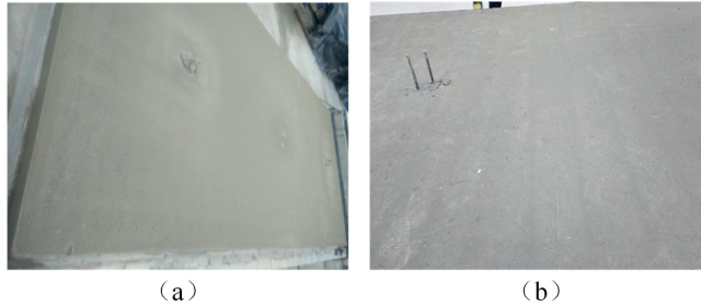
Fig. 17. Photographs of top surface of filing layer; (a) Mix No. 0.484-0.195-13.6; (b) Mix No. 0.616-0.197-12.4
