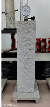
Fig. 3. Photograph of the drying shrinkage test
