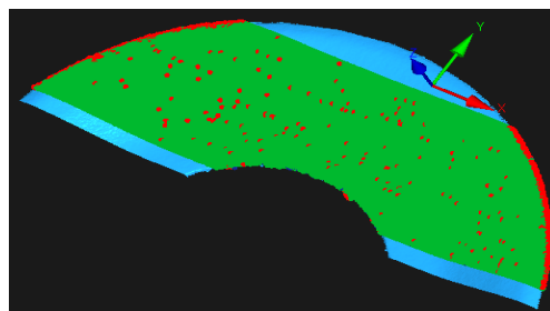
Fig. 5. View of the deviations in the ZRE software for the data measured by using the following parameters: v=1 mm/s, res=0.03 mm
