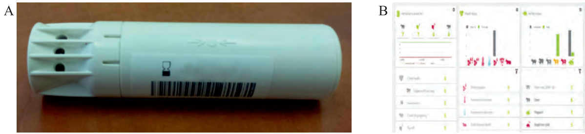
Fig. 2. SmaXtec system: bolus (sensor) (A) and SmaXtec messenger® computer software (B).
