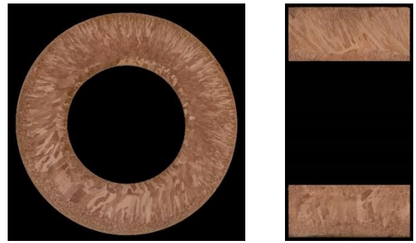
Fig. 5. Typical macrostructure of cast hollow rods \varnothing 45 \times 10.5 mm
