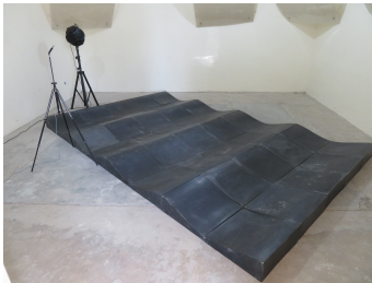
Fig. 3. Arrangement of the perforated panel in the reverberation chamber. The layout of the audio microphone and speaker.
