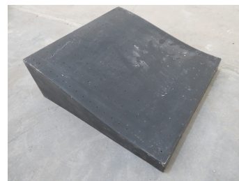
Fig. 2. Non-flat perforated panel (shape C) of 50 × 50 cm dimension.
