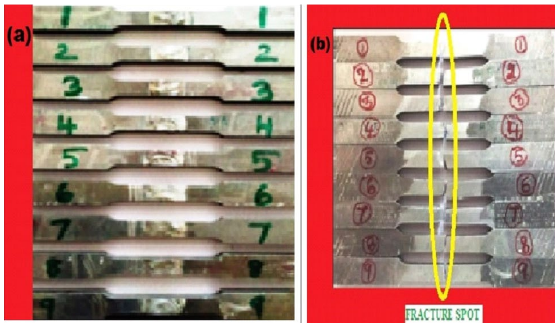
Fig. 3. (a) Tensile test specimens before tensile test; (b) Fractured tensile specimens after test
