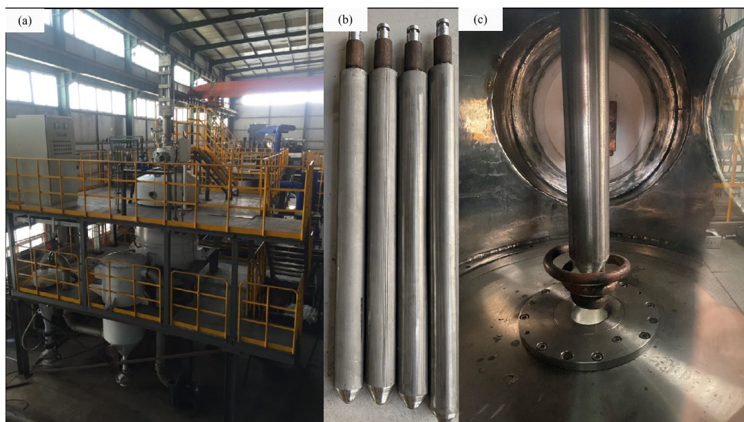
Fig. 1. Self-developed EIGA device; (a) EIGA device, (b) superalloy bar, (c) melting chamber
