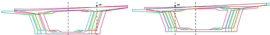
Fig. 2. Scheme of changing geometry of the superstructures; sections are marked with colours as follows: green marks a typical section, orange marks a section at the beginning of the structure, cyan marks a section with the maximum deviation to the right, red marks a section with the maximum deviation to the left, and purple marks a section at the end of the structure
