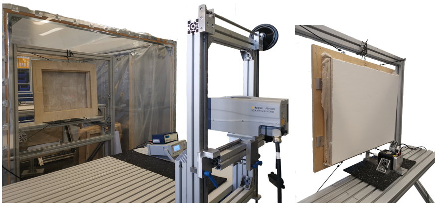
Fig. 3. The whole setup to conduct an experimental modal analysis of the dummy painting in a climate box with approximately free suspension
