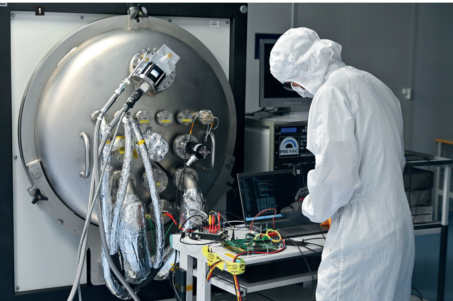
Photo 1 Thermal-vacuum chambers are set up in the clean room, which was commissioned for use in 2022
