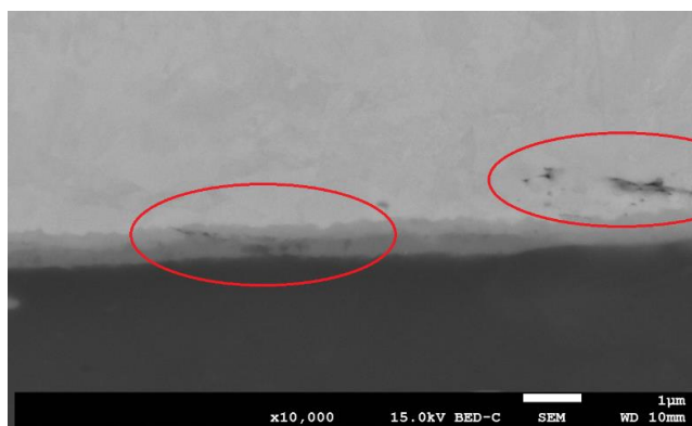
Fig. 8. Pores and voids due to oxide contamination, SEM image
