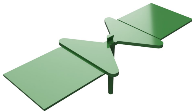
Fig. 1. 3D drawing of injection moulded parts with sprue
