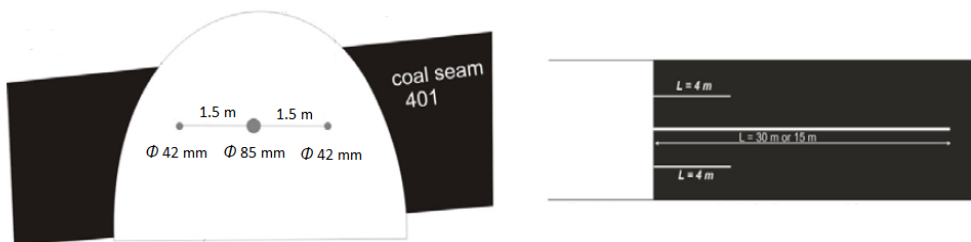
Fig. 6. Drilling layout for water injection tests in the roadway coal face in the 401 coal seam
