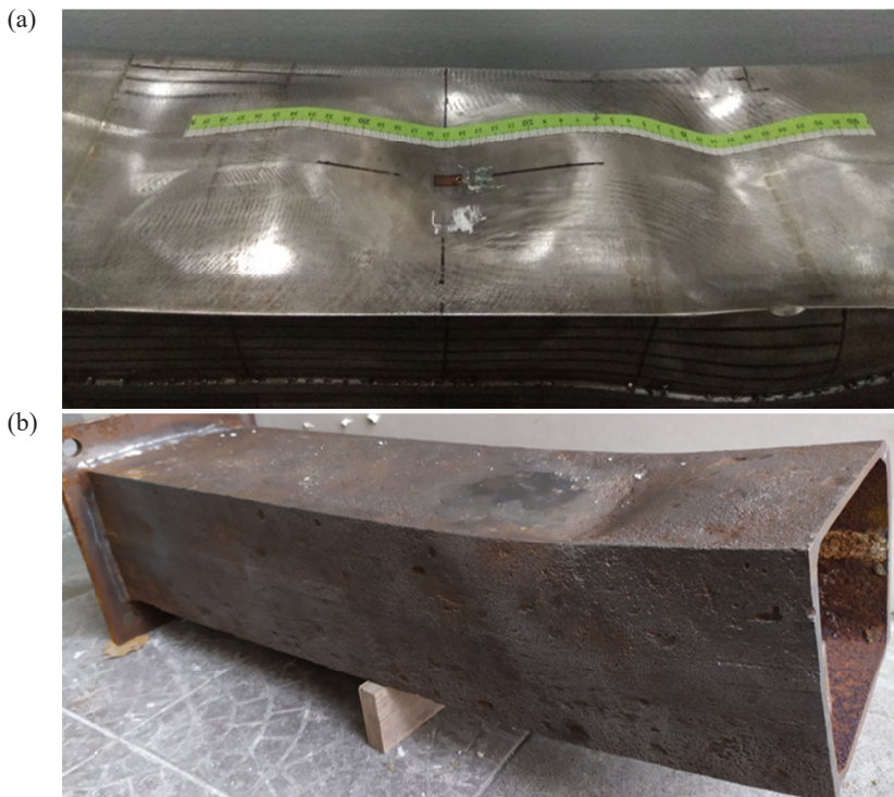
Fig. 7. Results of bending tests: (a) uniform, artificially corroded and (b) naturally corroded guide specimen
