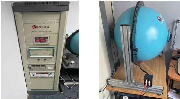
Fig. 5. View of the LPCE-2 spherical measurement system by Lisun Group.
