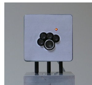
Fig. 11. Sonar module used in experiments.
