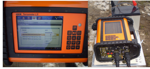
Fig. 11. View of the tomograph – Terrameter LS of the Swedish company ABEM [15]
