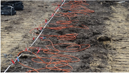
Fig. 10. A set of electrodes prepared for tomography examination in real conditions [15]
