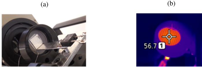
Fig. 5. Installation of a PV cell and a heating diode on a common heat sink (a), temperature distribution on the surface of the tested PV cell (b).
