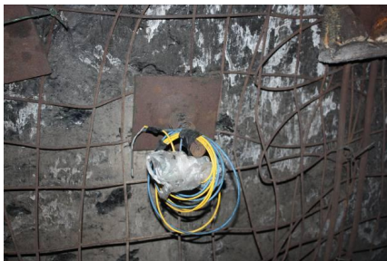
(b) Rebar bolt with optical fiber
