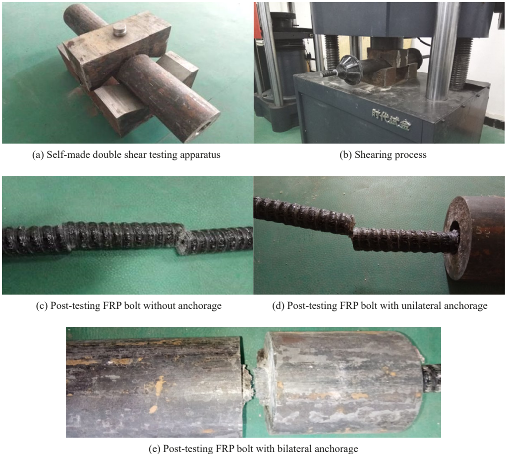
Fig. 8. Shearing test of FRP bolts under different anchorage conditions
