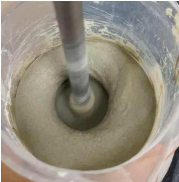
Fig. 2. Doughnut formation during geopolymer mixing
