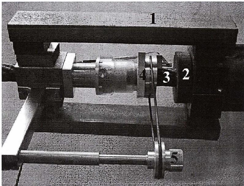
Fig. 4. Measuring head GPW (measuring head with the rotating sensor)
