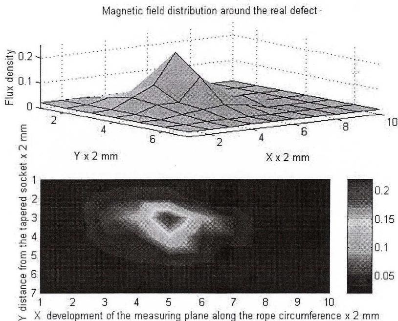
Fig. 7. Distribution of stray field induction around the defect
