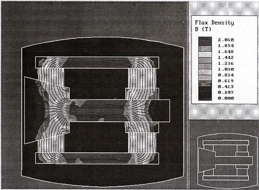
Fig. 5. Magnetic field distribution in the magnetic circuit
