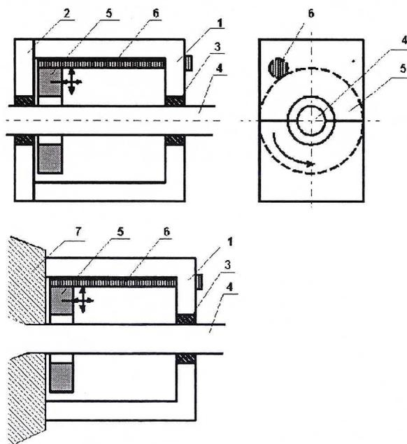
Fig. 3. New instrument for inspecting rope ends in tapered sockets
