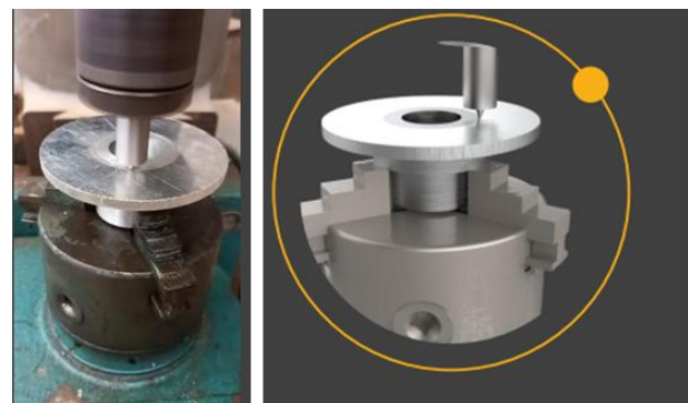
Fig. 3. Shows the fixture and set used to induce FSW for a flange in schematic form
