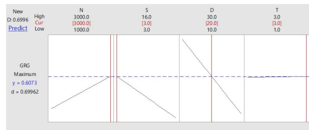
Fig. 15. Shows optimizing the factors and replies using the ANOVA response optimizer
