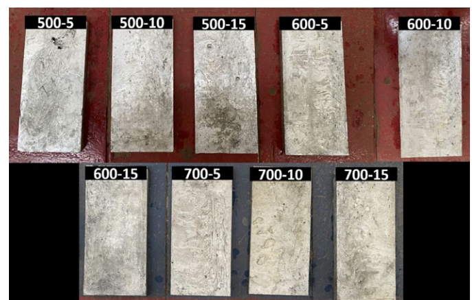
Fig. 2. Fabricated A713-2% TiB 2 MMCs
