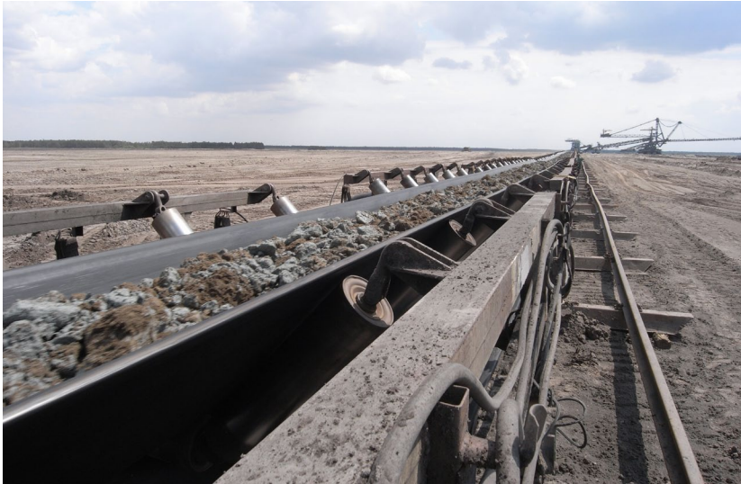
Fig. 1. The example of working belt conveyor in the open-pit mine ( Source : private archive)
