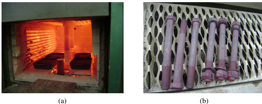
Fig. 1. Bolt soaking process: (a) inside the furnace chamber right after inserting the samples, (b) bolts of the same series: “bare” – for the shear test and provided with 2 washers and a nut – for the tensile test
