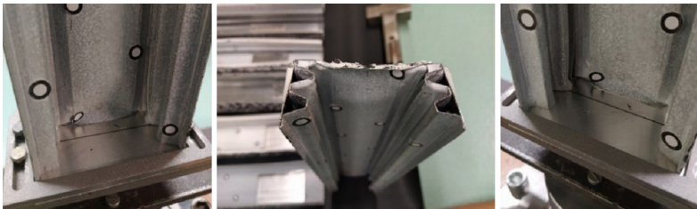
Fig. 8. Columns after performed tests
