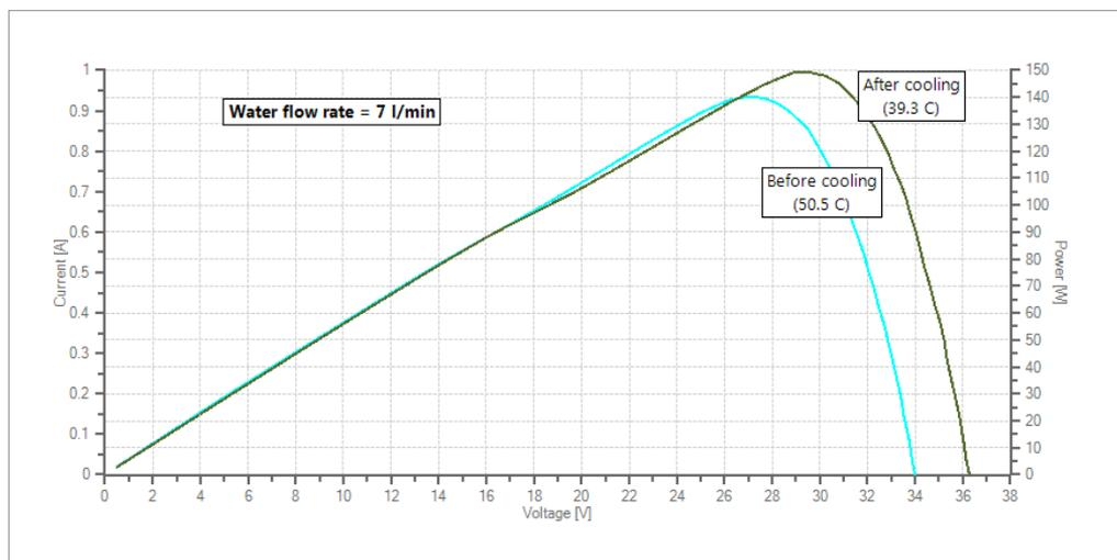
Fig. 7. PV power curve before and after cooling at 7 L/min water flow rate (CASE 3)
