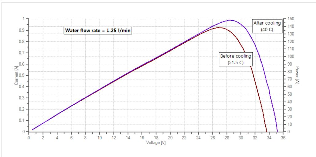
Fig. 5. PV power curve before and after cooling at 1.25 L/min water flow rate (CASE 1)
