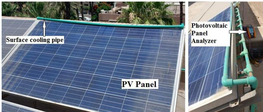
Fig. 4. Experimental PV panel setup
