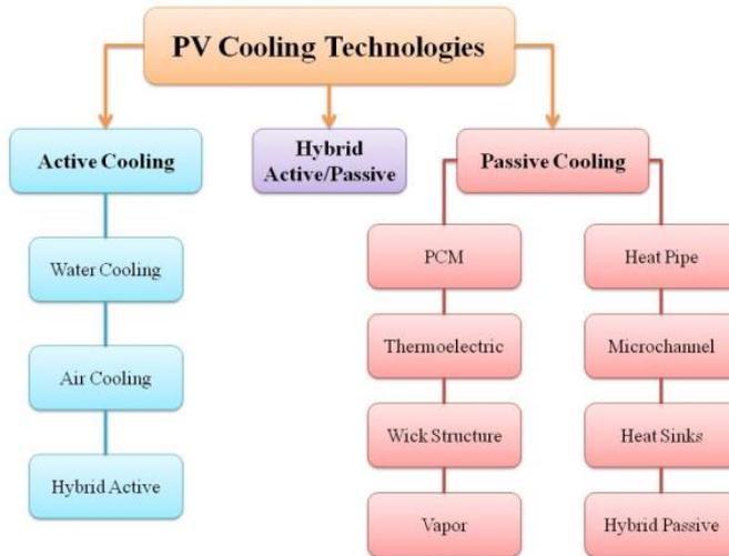
Fig. 2. Block diagram of PV cooling technologies (Shaaban et al. 2023)
