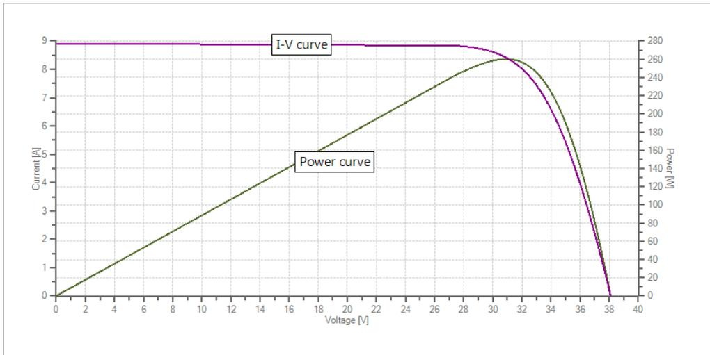
Fig. 3. IV and power curves of the PV panel
