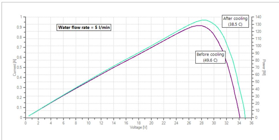
Fig. 6. PV power curve before and after cooling at 5L/min water flow rate (CASE 2)
