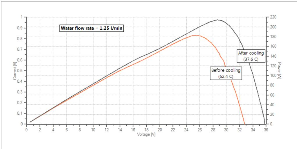
Fig. 9. PV power curve before and after 8 minutes of cooling at 1.25 L/min water flow rate
