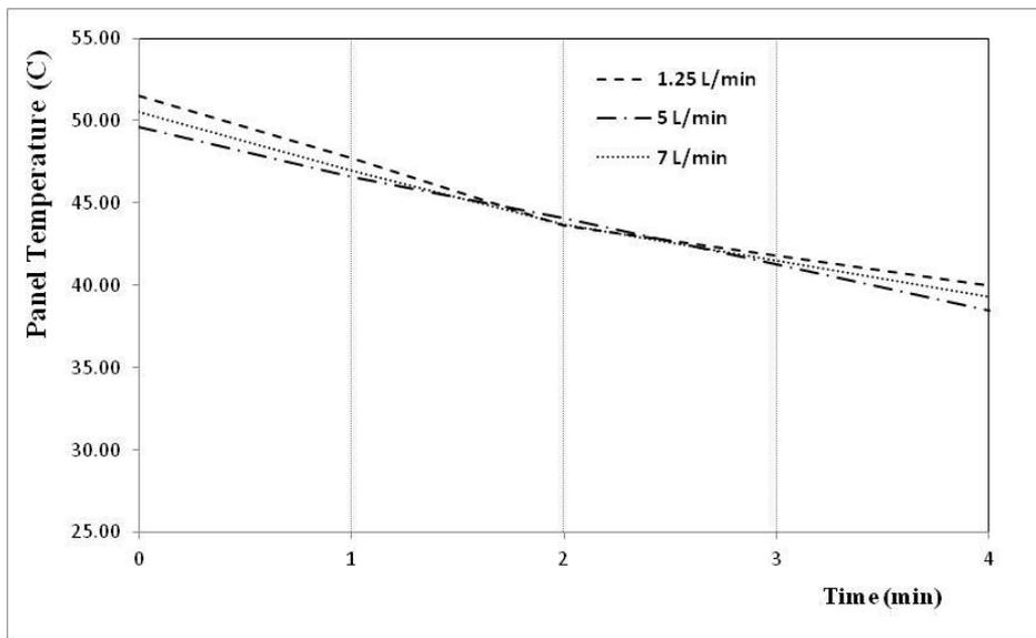
Fig. 8. PV panel temperature versus time at different water flow rates
