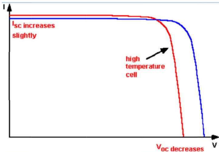
Fig. 1. Effect of temperature on PV characteristics (Panda et al. 2023)
