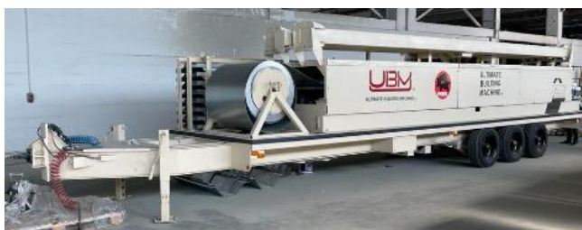
Fig.3. Prefabrication UBM machine.
