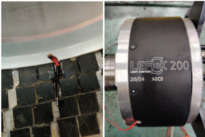
Fig. 6. Temperature sensors mounted on permanent magnets and placed outside the rotor
