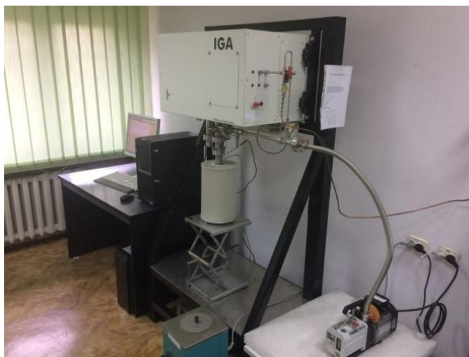
Fig. 4. IGA-001 gravimetric sorption system for methane sorption kinetics investigation
