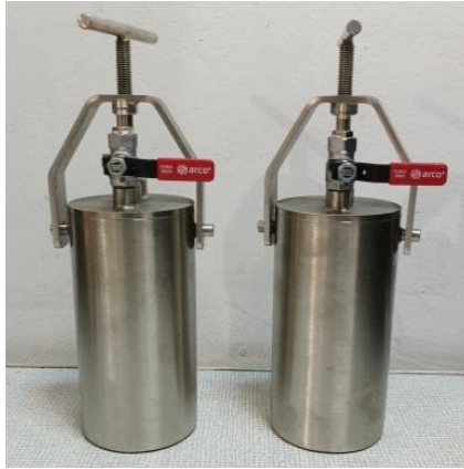
Fig. 2. Hermetically sealed containers for coal sampling
