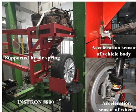
(a) McPherson test bench.
