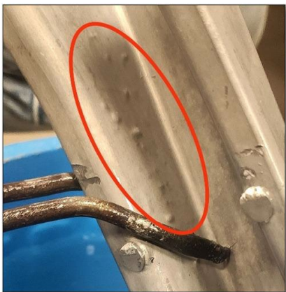
Fig. 1. Exemplary pressure die cast with visible blistering [own study]
