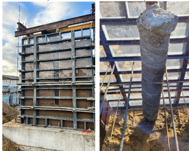
Fig. 6. Photographs of field research stand for pile load test: a) Transparent chamber filled with soil; b) pile used in the investigations [30].
