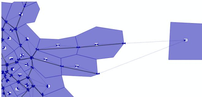
**Fig. 9.** Part of the model showing how zones are connected to links.
